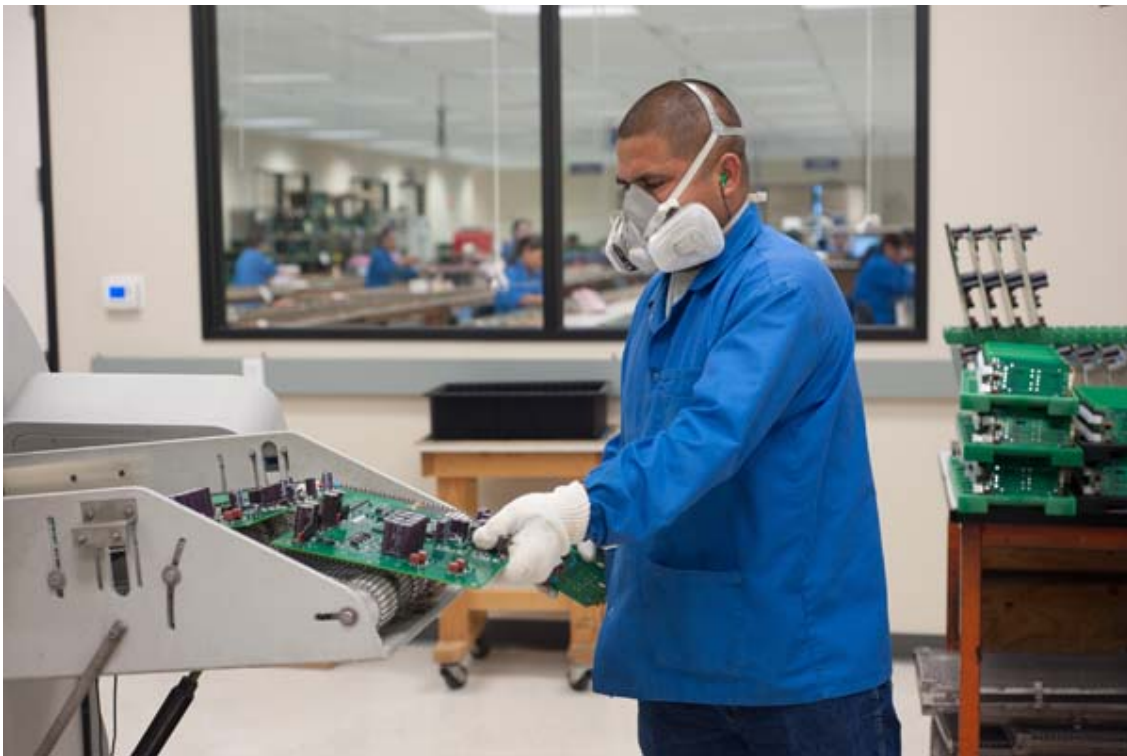
A technician at Bestronics carefully observes wave soldering of PCB assemblies Photo courtesy of Bestronics Inc., San Jose, California
